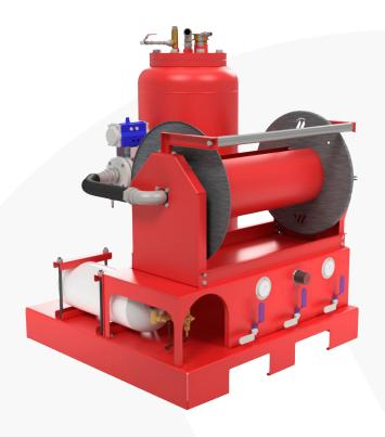
The construction materials of the hose reel's swivel joint of is made of antifriction material such as bronze with composite seals **VITON** + **PTFE** with internal passages of **1"1/2**, with very low pressure losses gather to the study of internal fluid dynamics carried out by **MALECO**.
